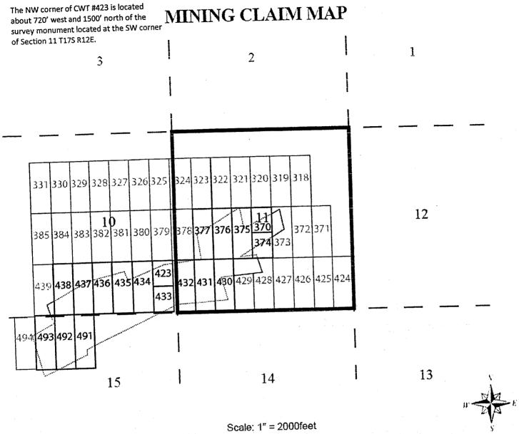
The above map depicts the \_\_\_\_\_ CWT #423 \_\_mining claim, which is located in Section (s) \_\_\_\_\_ 10 \_, Township 17 South , Range 12 East , Gila and Salt River Base and Meridian, Pima County, Arizona. The types of corner and location monuments used are as follows: Rock and Post. All claims depicted on the map are 1500 feet between each end and 600 feet between each side. The bearings between all claim corners are north-south and east-west as depicted on the map.
