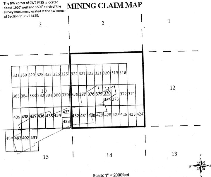
The above map depicts the \_\_\_\_\_ CWT #435 \_\_mining claim, which is located in Section (s) \_\_\_\_\_, Township 17 South , Range 12 East , Gila and Salt River Base and Meridian, Pima County, Arizona. The types of corner and location monuments used are as follows: Rock and Post. All claims depicted on the map are 1500 feet between each end and 600 feet between each side. The bearings between all claim corners are north-south and east-west as depicted on the map.
